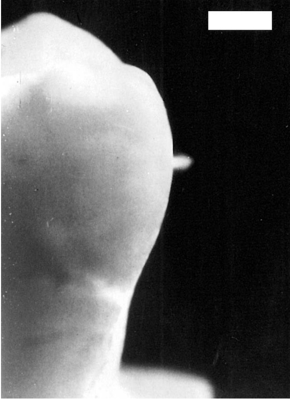
Fig. 3.40. Laser-induced plasma sparking on tooth surface caused by a single pulse from a Nd:YLF laser (pulse duration: 30 ps, pulse energy: 1 mJ, focal spot size: 30 \mu m, bar: 1 mm). With these parameters, a power density of about 5 \times 10^{12} W/cm 2 is obtained
